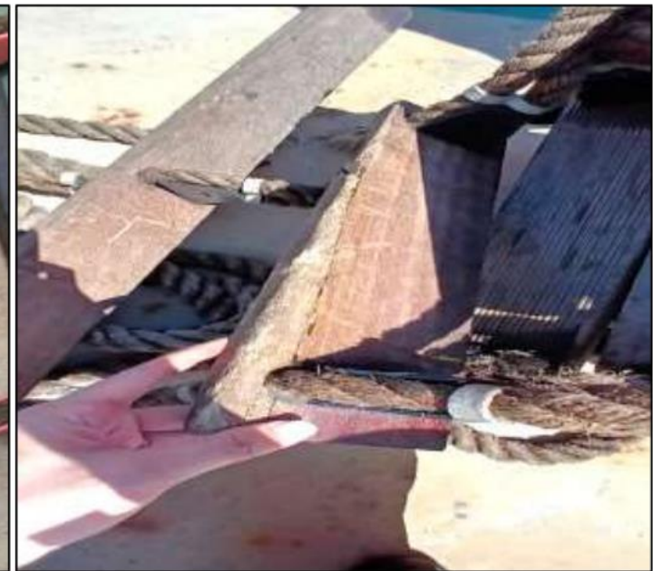
Pilot ladder no. 2 - Deformed pilot ladder step
