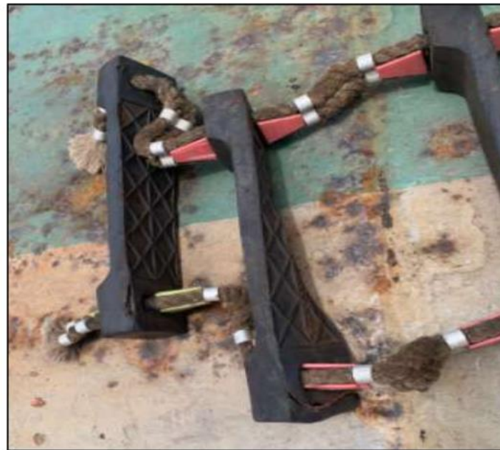
Pilot ladder no. 1 - Cracked pilot ladder step
