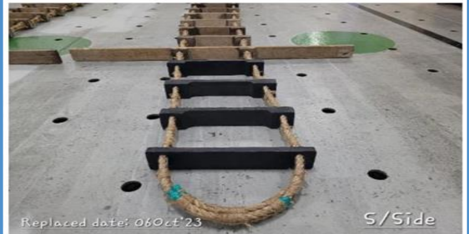
Starboard Side Pilot Ladder (Bottom Section)
