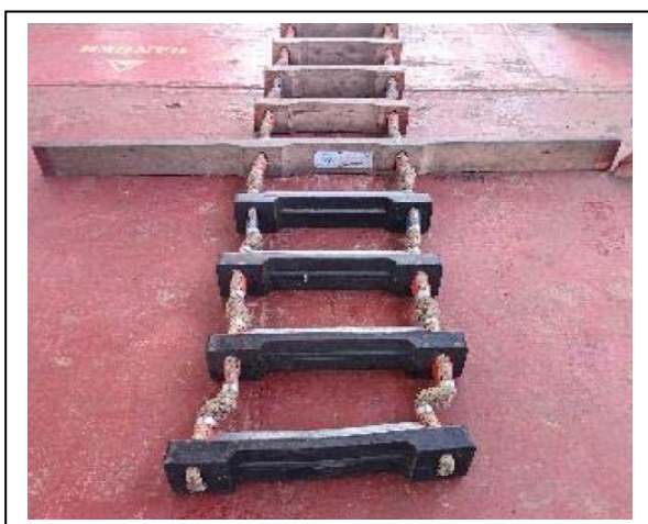
“Non-compliant ‘bottom’ and ‘top’ construction of a pilot ladder”
