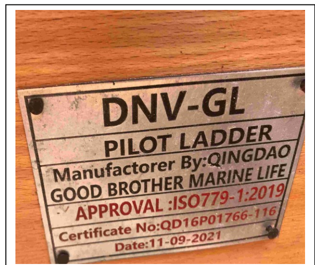
Certificate and identification tag for a counterfeit pilot ladder
