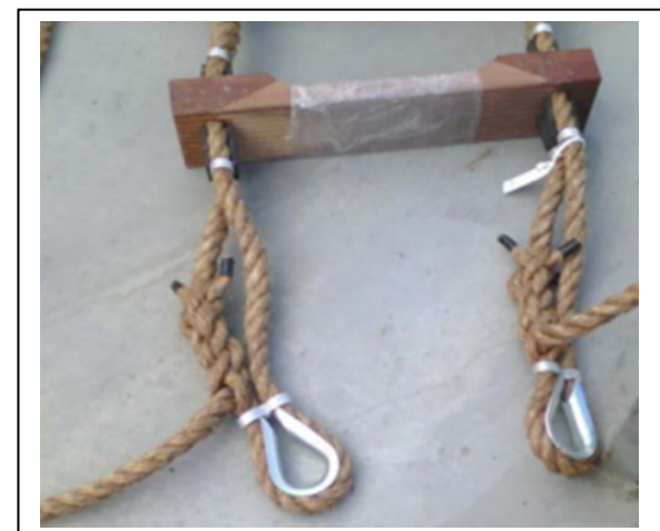
“Non-compliant ‘bottom’ and ‘top’ construction of a pilot ladder”
